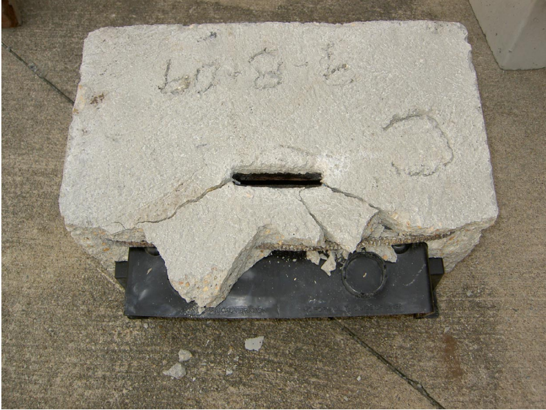
Figure B-7. Bottom View: cracking (rupture) of rebar-reinforced SmartSlope block at the completion of a connection test
