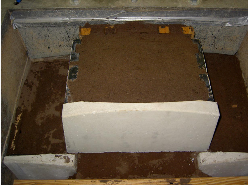
Figure B-3. Sand nominally compacted within and between SmartSlope Blocks.
