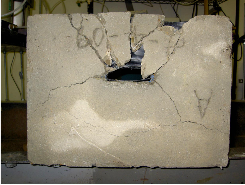
Figure B-5. Bottom View: cracking (rupture) of SmartSlope block at the completion of a connection test
